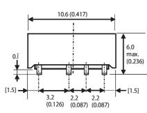
Tolerance of lead pitch is  $\pm 0.15$ mm (0.006inch) Other tolerances  $\pm 0.3$ mm (0.012inch)
