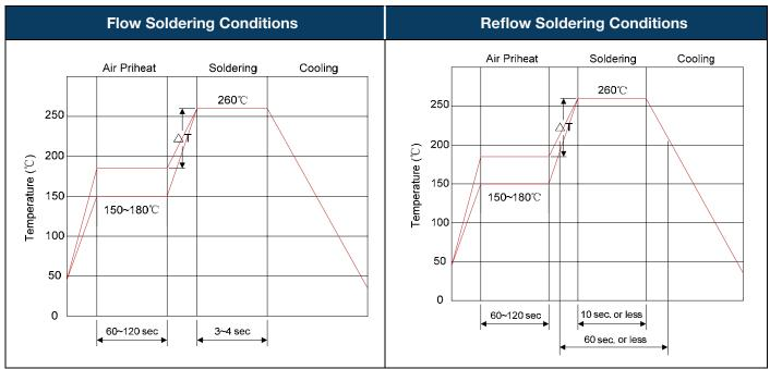
1) Time shown in the above figures is measured from the point when chip surface reaches temperature.
