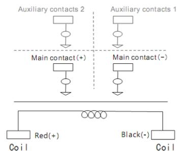
Coil extraction mode: UL3266 、 20AWG 、 320±20mm (Connectors can be configured by the customer)
