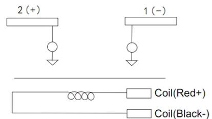
Coil extraction mode: UL3266 、 20AWG 、 320±20mm (Connectors can be configured by the customer)
