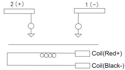
Coil extraction mode: UL3266 、 20AWG 、 320±20mm (Connectors can be configured by the customer)
